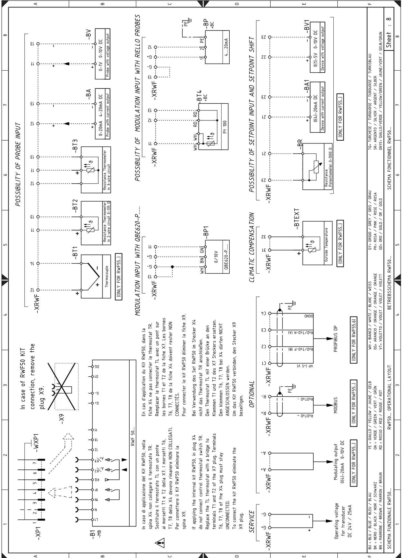
In case of RWF50 KIT connection, remove the plug X9.
