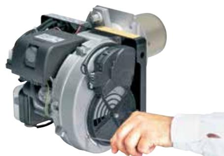
Head setting is easy and aided by a graduated scale, a test point allows reading the air pressure in the combustion head.
