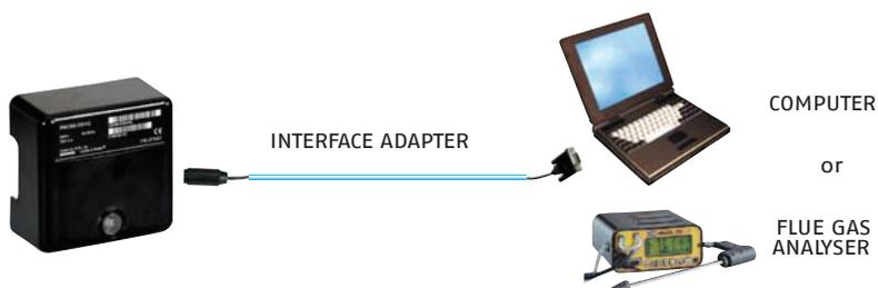
by the interface adapter and a PC with dedicated software or by a predisposed flue gas analyser (see paragraph accessories).
