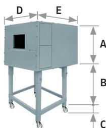
If noise emission needs reducing even further, sound-proofing boxes are available. In case of generator heights, where a lower dimension "B" is required, ask for the Box Support Kit code 20065135. The useful dimensions are 40 mm less than the total dimensions indicated in the table (A, D, E). Not suitable for outdoor use.
