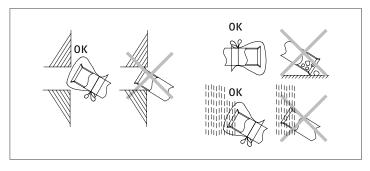
A Before threading the lines through the hole in the wall, close the lines ends.
