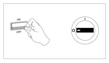
— position the system's main switch in the "OFF" position. To access the terminal board:
