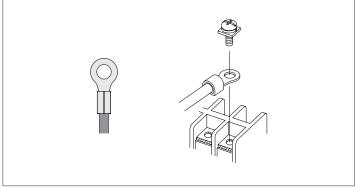
It is compulsory to use ring crimp terminals to connect to the terminal board.
