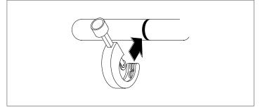
— cut the pipe end square using a pipe cutter
