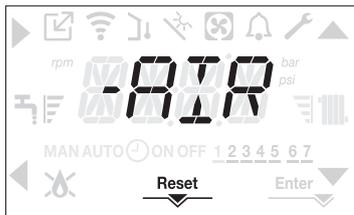
Press the RESET button to interrupt the venting cycle. Turn the boiler OFF by pressing
