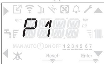
Access to parameter programming of the TECHNICAL menu is protected by a password; by pressing MENU again for at least 2 seconds, the letters PWD will flash for 2 seconds (0.5 sec ON and 0.5 sec OFF).
