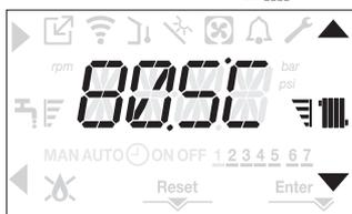
If button C or D is pressed and held, the meter will alter the set value more quickly. If no button is pressed for 5 seconds, the set value is taken as the new heating setpoint and the display returns to the main screen.
