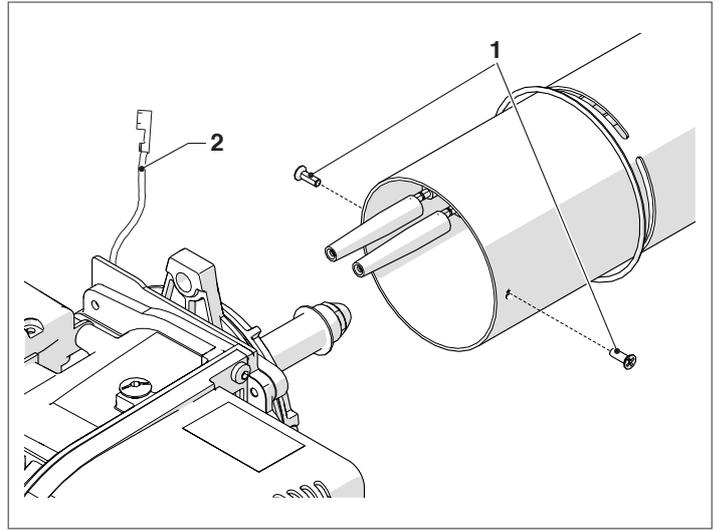
**⚠** With the blast tube removed, check its front edge to make sure that it is smooth, free from deposits, burns and dents.
