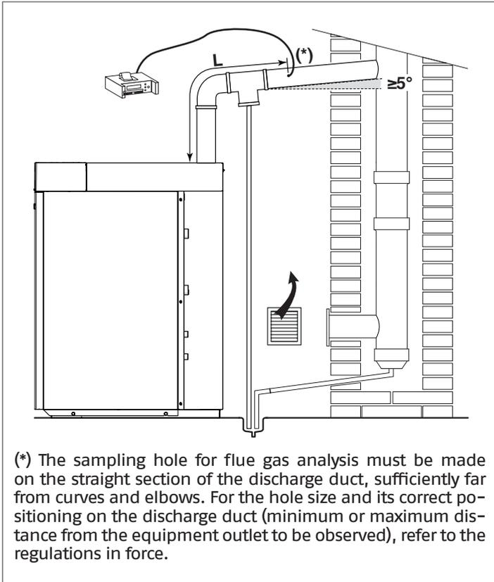
(\*) The sampling hole for flue gas analysis must be made on the straight section of the discharge duct, sufficiently far from curves and elbows. For the hole size and its correct positioning on the discharge duct (minimum or maximum distance from the equipment outlet to be observed), refer to the regulations in force.
