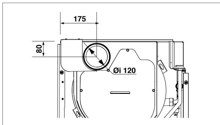
**INSIEME EVOe 32 V LN** boilers derive their comburent air from the room in which they are installed. Suitable air vents must therefore be provided in compliance with applicable laws and standards.
