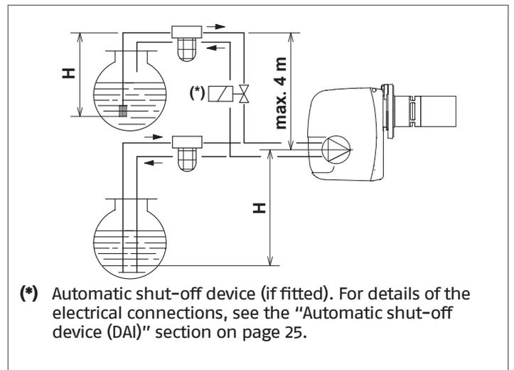
**⚠** If a confirmation solenoid valve is to be installed in the light oil supply circuit to the burner, only a one-pipe system can be set. Any two-pipe connection can compromise the correct operation of the burner.
