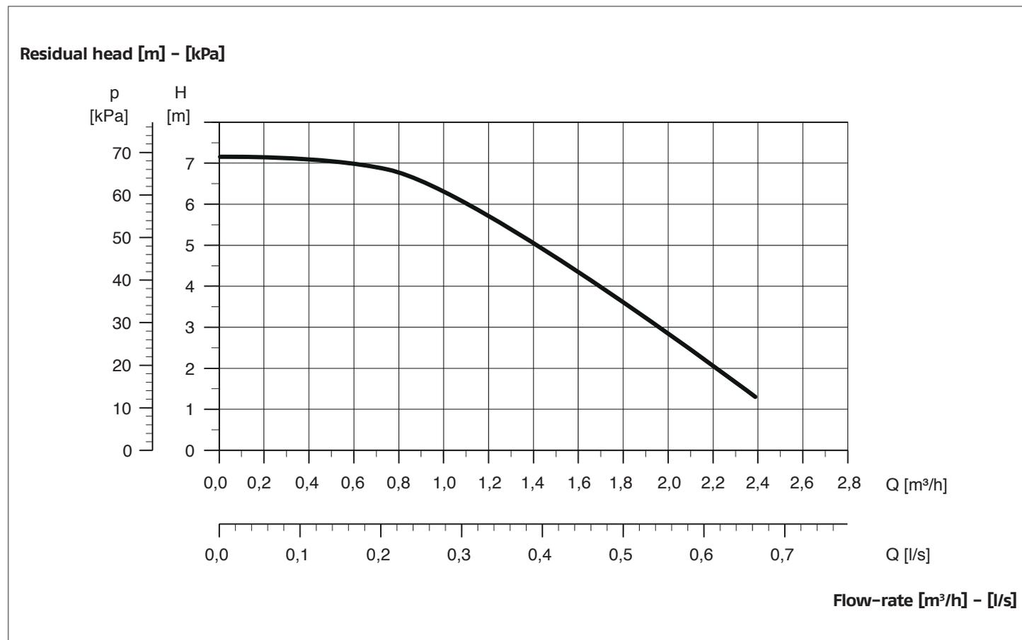
The curves refer to a density of 983.2 Kg/m<sup>3</sup>, a water temperature of +20°C and a kinematic viscosity of 0.474 mm<sup>2</sup>/s (0.474 cSt).
