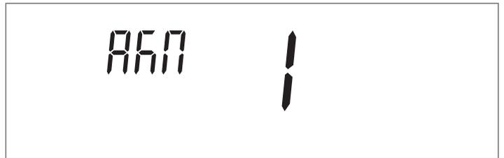
At first start-up and at every restoration of the power supply the venting function signalled by the message "Air" activates. The vent cycle lasts 14 minutes.
