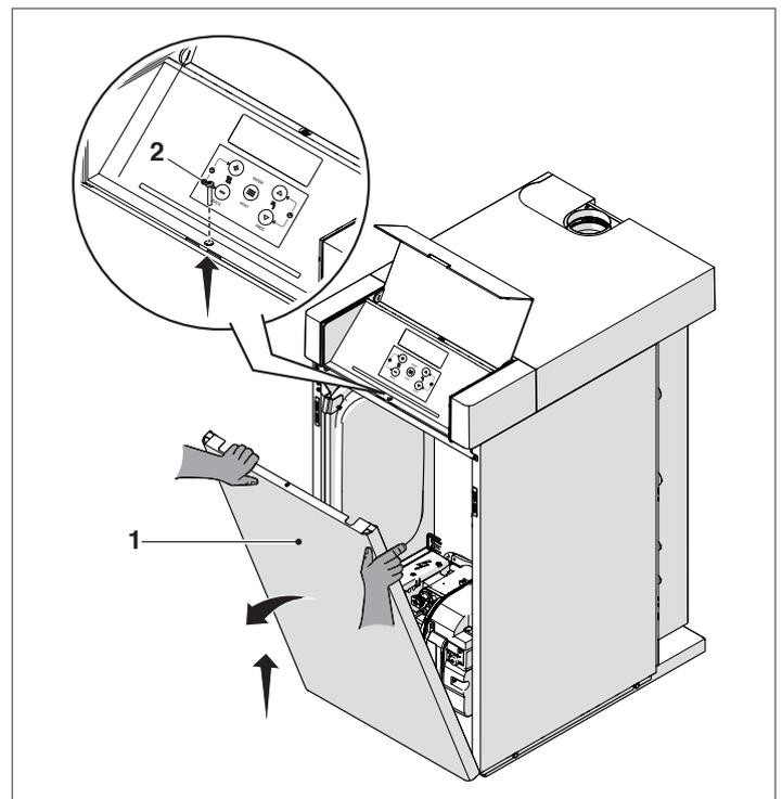
**REMOVING THE BURNER**
