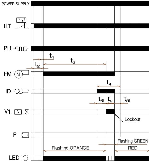
Lockout caused by extraneous light during pre-purging
