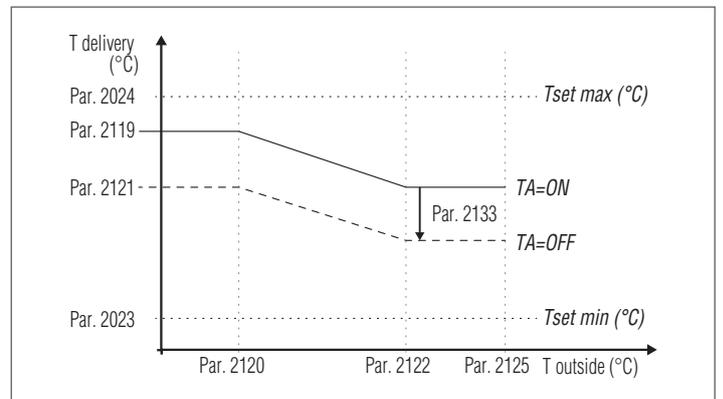
**⚠** If the external probe (accessory) is not detected (not installed or damaged), the system makes a heat request at the maximum setpoint set on the climatic curve.
