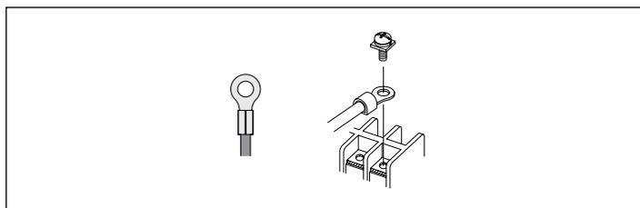
**⚠** It is compulsory to use ring crimp terminals to connect to the terminal board.
