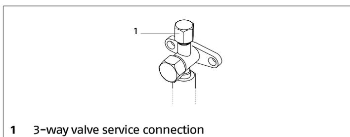
— charge the circuit with nitrogen through the service connection on the 3-way shut-off valve
