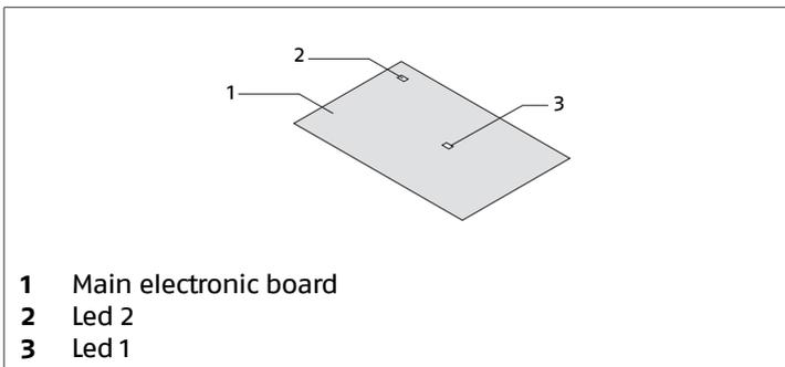
The unit operation is signalled with LED 2.
