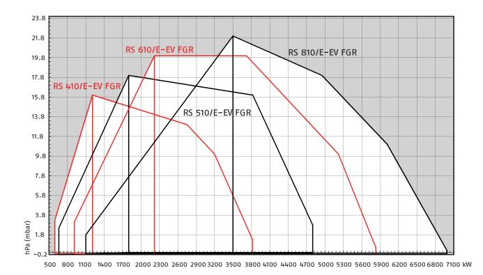
Test conditions conforming to EN676 Temperature: 20°C Pressure: 1013,5 mbar Altitude: 0 m a.s.l.
