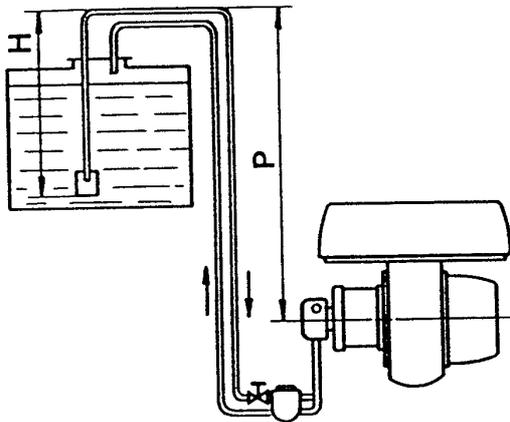
The dimension P should not exceed 10 m, to avoid breakage of pump seals.
