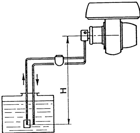
Oil lines must be perfectly sealed. The use of copper pipe is therefore recommended. The pump suction must not exceed 4 m w.c. (30 cm Hg) because beyond this value the pump becomes noisy.
