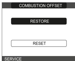
**RESTORE:** select this option when replacing the MAIN PCB electronic board
