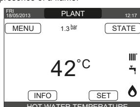
The boiler will be in function until the selected temperature is reached, afterwards it will be in "standby" again keeping the outlet temperature displayed. If faults arise in ignition or operations, the boiler performs a "SAFETY STOP": the triangle signalling faults will flash on the REC10CH. To identify the fault codes and to reset the appliance, see the section "4.14 Lights and faults".
