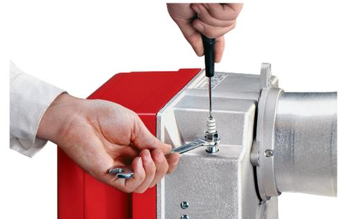
Head setting is easy and aided by a graduated scale; a test point allows reading the air pressure in the combustion head.
