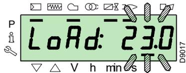
To exit manual mode, press the keys "+" and "-" (ESC) simultaneously for 3 seconds: the burner will work in Automatic mode and the output will depend on the thermostat/adjustment pressure switch (TR).
