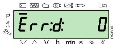
The burner goes into lockout.
