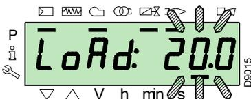
Releasing the "F" key, the standard visualisation appears, with the current load percentage flashing: this means that the burner is working in Manual mode (any outside adjustment is excluded and only the safety devices are active).
