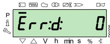
The burner goes into lockout.
