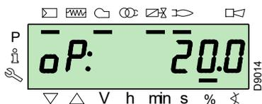
Press the “F” key for 1 second: “LoAd” is displayed and the load percentage flashes.
