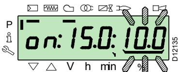
Select another point, or exit this area by pressing the keys "+" and "-" (**ESC**) simultaneously.
