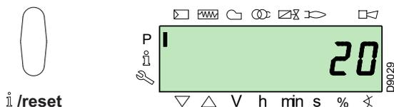
Press the key "+" and increase the value to 25 seconds (flashing). Press the key "i/reset" to confirm and store.
