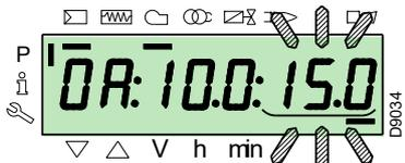
To adjust the speed of the inverter (expressed in % and that is **50 Hz = 100 %**), keep the buttons "F" and "A" simultaneously pressed, the percentage position blinks and press buttons "+" or "-" to increase or decrease the value.
