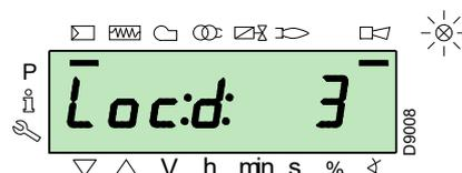
The display visualises alternately an error code and a diagnostic, which does not take the system into safety mode.
