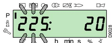
If the value is not visualised, press the key "i/reset" for 1 - 3s. An example of how to modify the parameter relating to **pre-purging time** (no.225) is given below. Press the key "i/reset": the value 20 (seconds) will appear.
