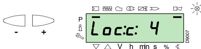
Confirm with the key "i/reset". The burner starts up.
