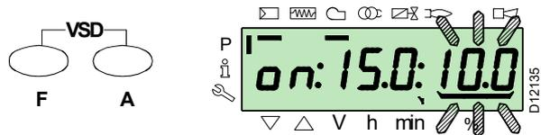
Select another point, or exit this area by pressing the keys "+" and "-" (ESC) simultaneously.
