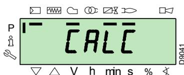
The control box will automatically calculate the points from "P8" to "P2", distributing them in a line. These are theoretical and must be checked.
