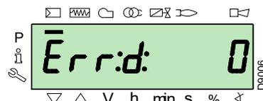
The burner goes into lockout.
