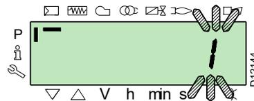
confirm with the button "i/reset" to activate the **backup** process.
