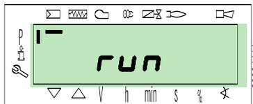
Confirm with the key "i/reset". The burner starts up.
