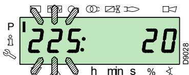
If the value is not visualised, press the key "i/reset" for 1 - 3s. An example of how to modify the parameter relating to **pre-purging time** (no.225) is given below. Press the key "i/reset": the value 20 (seconds) will appear.
