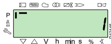
After approx 5 seconds (it depends on the duration of the programme), the 0 value appears on the display screen, this is to indicate that the backup process has been completed correctly.
