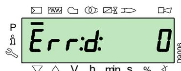
The burner goes into lockout.
