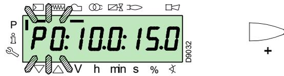
Access the Parameters Level referring to "Access procedure with password" at page 41. The display screen displays the parameters group 400.
