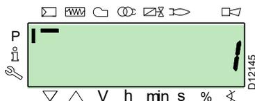
After approx 8 seconds (it depends on the duration of the programme), the 0 value appears on the display screen, this is to indicate that the restore process has been completed correctly.
