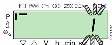
confirm with the button "i/reset" to activate the **restore** process.
