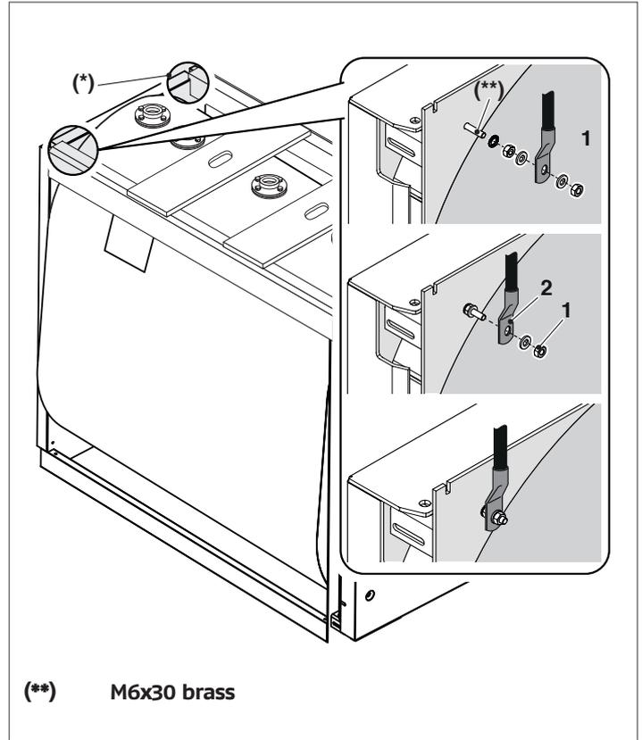
**!** Another hole (\*) in the left side of the boiler head can also be used to earth the appliance. If you wish to use this hole for the earth connection, remove the terminal fittings from the right of the head and move them to the left earthing point.
