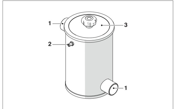
**!** It is mandatory to check and clean the condensation trap and pipes, up to the collection/drain point, at least once a year.
