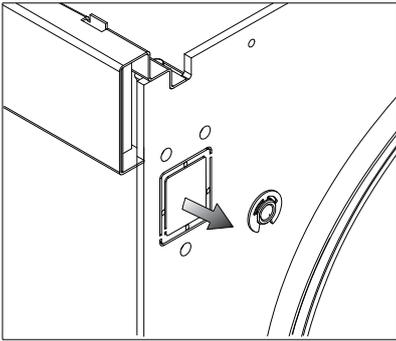
Open the door and with the aid of a small hacksaw or a file remove the knockout on the side opposite the leading edge of the door (both top and bottom).
