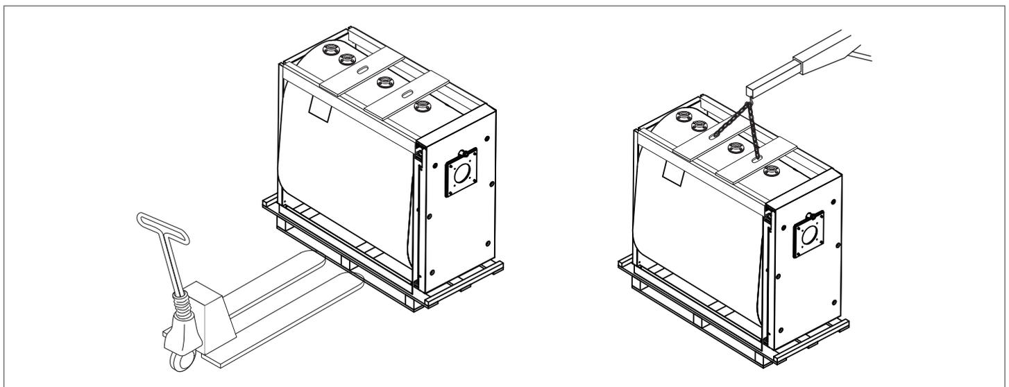
**TAU N OIL PRO RIELLO** steel boilers are fitted with lifting attachments. Take great care when moving them and only use lifting equipment of adequate capacity.
