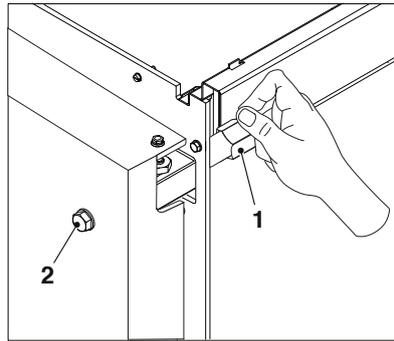
Then seal the door by tightening the bolts (2) so that the door is self-supported by compression against the packing. Remove the plug (1) taking care not to lose the compressed spring inserted in the threaded tube.
