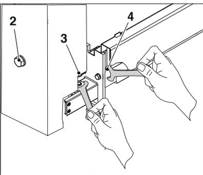
Remount the hinge plate on the opposite side, ensuring that the cylinder projecting above the nut (6) enters into its slot. If necessary tighten the nut (6) to raise it. Lastly, tighten the bolt ((3)).
