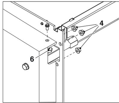
Remove the nuts (4) that secure the hinge plate (5) to the door and remove the plate.
