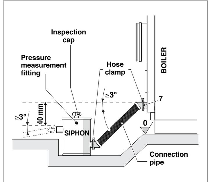
**⚠** Before commissioning, fill the siphon with water up to level "L" in line with the top fitting.
