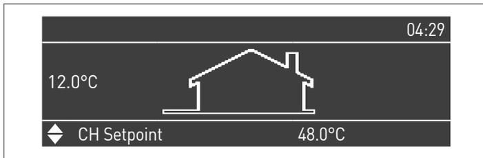
External temperature is shown on the display on the left. This value is displayed only if the outdoor temperature sensor (accessory) is installed.
