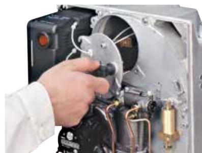
The 7-pole socket is incorporated in the control box, the 4-pole socket is already connected.
