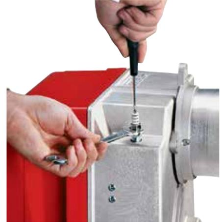
1st stage air damper position adjustment.
