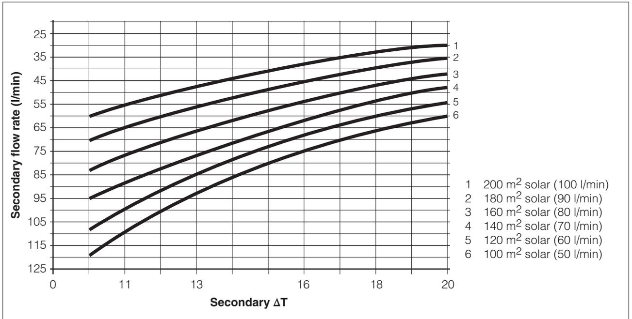
**NB:** Assuming primary circuit parameters 0.5 l/min\*m<sup>2</sup> -  $\Delta T$  12 °C (95 °C to 83 °C) / Secondary circuit flow 90 °C
