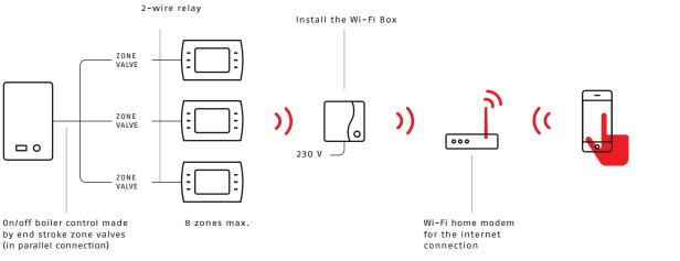
NB: When replacing an old thermostat that has more than two wires, identify the 'switch' wires and connect only them to the RiCLOUD ON/OFF terminals (do not connect a Neutral supply to RiCLOUD). The RiCLOUD control is powered by batteries; it therefore does not require a fixed mains power supply.
