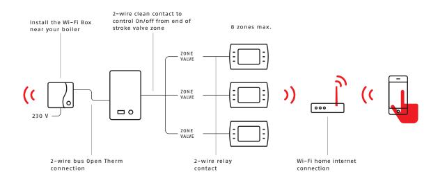
NB: When replacing an old thermostat that has more than two wires, identify the 'switch' wires and connect only them to the RiCLOUD ON/OFF terminals.
