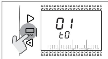
Press the FORWARD > or BACK < button to select the desired parameter.
