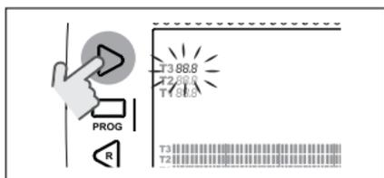
Press the UP ^ or DOWN v button to modify the selected room setpoint temperature.
