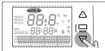
Press the SET/PROG button to save and return to the HOME screen, press ESC/MODE to save and return to the HOME screen, or wait 5 seconds to automatically save the value and return to the HOME screen.
