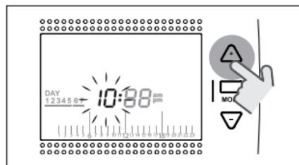
Press the SET/PROGRAM button to save and return to the programming menu, press ESC/MODE to save and exit the programming menu, or wait 30 seconds to automatically save the value and return to the home screen.
