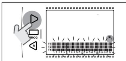
Press the SET/PROG button to set. Press the FORWARD > or BACK < button to select the day or period of the week to be changed.
