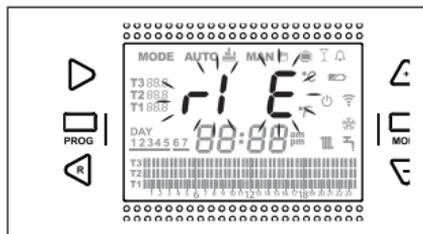
press the ESC/MODE button and hold for 5 seconds to start semi-automatic filling (the message rIE will stop flashing and remain on). When releasing the button ESC/MODE the rIE message starts flashing slowly (2 secs) until the end of the function.
