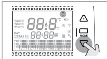
The room temperature set cannot be less than or equal to the desired T3 (comfort) room setpoint temperature.
