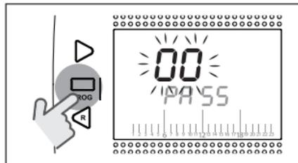
Press the UP ^ or DOWN v button to insert the installer password (password = 18).
