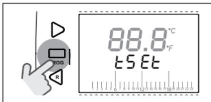
Press the UP ^ or DOWN v button to select the desired parameter and wait until it is displayed.
