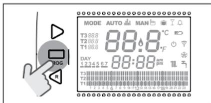
Press the FORWARD > or BACK < button to select the field DHW TIME PROGRAM
