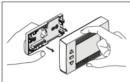
Fix **RiCLOUD** base to the wall or electrical box using the screws provided, use the optics level in the plastic wrapping to install **RiCLOUD** horizontally.
