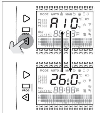
In case of a boiler alarm (available with OTBus connection between the WiFi Box and the boiler, if provided for by the OTBus protocol), the alarm can be reset by pressing the BACK/RESET button < (for alarm A99, reset from the boiler).
