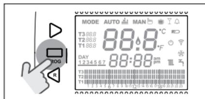
Press the FORWARD > or BACK < button to select the field HEATING/Cooling TIME PROGRAM.
