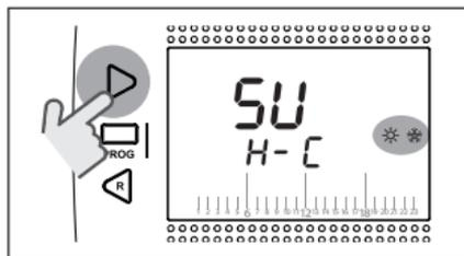
Press the SET/PROG button to save and return to the programming menu, press ESC/MODE to save and exit the programming menu, or wait 30 seconds to automatically save the value and return to the HOME screen
