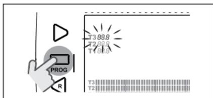
Press the FORWARD > or BACK < button to select the temperature to be changed.
