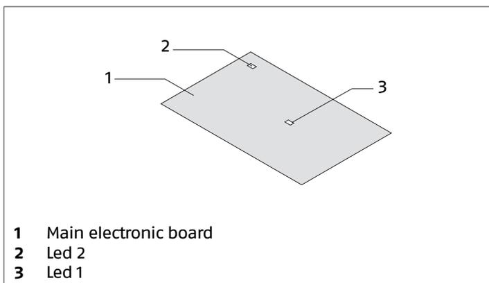
The unit operation is signalled with LED 2.
