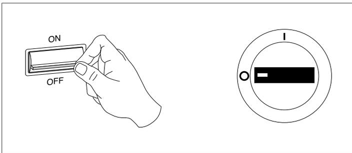
**⚠** Wait 10 minutes before touching the device electric components.
