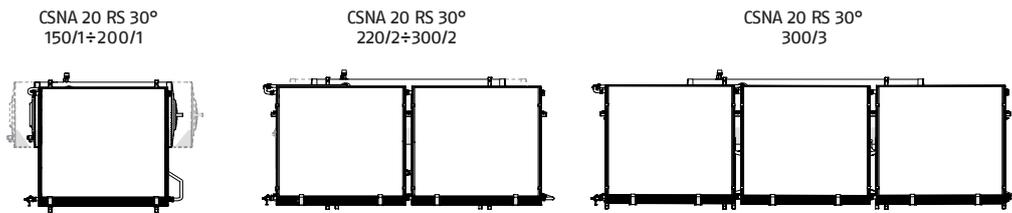
**SYSTEM STRUCTURE CSNA 20 RS 0° (installation on pitched roofs) system layout**
