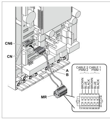
Connect the PWM controls of the pumps to the feedback terminal board (MR).
