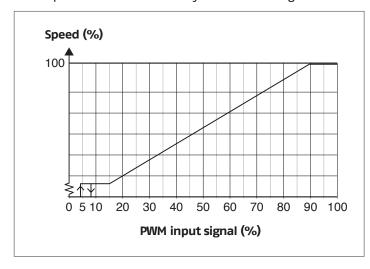
A Verify that the control logic of your pump is directly proportional (as indicated in the chart) and not inversely proportional.
