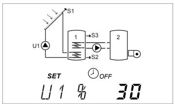
NOTE: With NON modulating pumps, "100" is displayed when the pump is stopped and "0" when the pump is operating.
