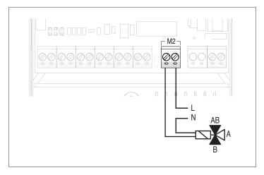
The regulator only manages non-modulating on-off valves. The connection to the CN6 connector must not be used.
