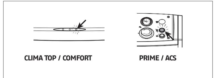
**!** If a "LOCKOUT SHUTDOWN" occurs, wait about 30 seconds before resetting the burner.
