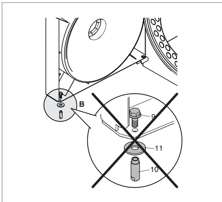
**⚠** The first time you open the door, remove the spare hinge assembly 'B' [bushing (10), bolt (9), and washer (11)] opposite the hinged side of the door.
