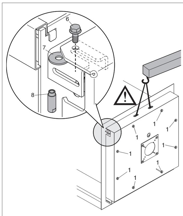
**⚠** If it proves difficult to fit the washer (7) or screw the bolt (6) into the bush (8) because the door is not accurately aligned, **attach a hoist of adequate lifting capacity to the door** (see the weights and dimensions table), **slightly loosen** the fixing bolts (1) and lift the door just enough to fit the washer (7) or align the hole in the door with the hole in the hinge. **Once the bolt (6) has engaged the bush, re-tighten the door fixing bolts (1).**
