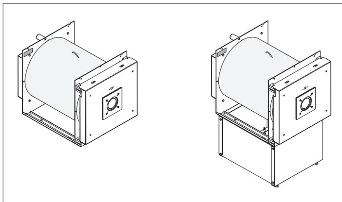
**⚠** If you are installing the boiler without a pedestal, the limited gap between the burner and the floor makes it particularly important to keep the boiler room clean.
