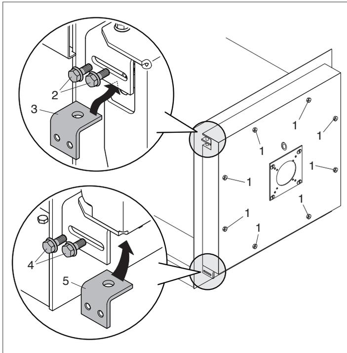
**⚠** Make sure that the safety bolts (2 and 4) are securely tightened before attempting to open the door.
