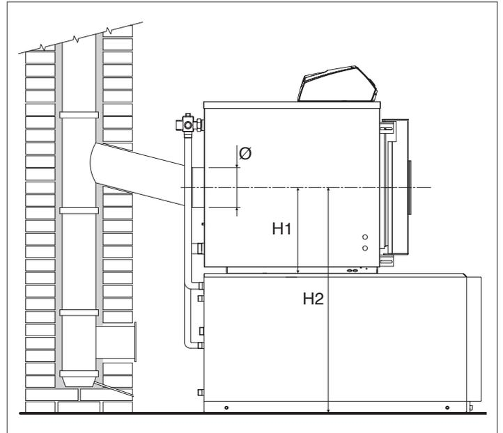
**⚠** The stack must guarantee the minimum draught specified by applicable technical standards, assuming zero pressure at the connection to the flue gas exhaust. Draught at the stack must not exceed 0.2 mbar. Fit a draught limiter if draught exceeds this value.
