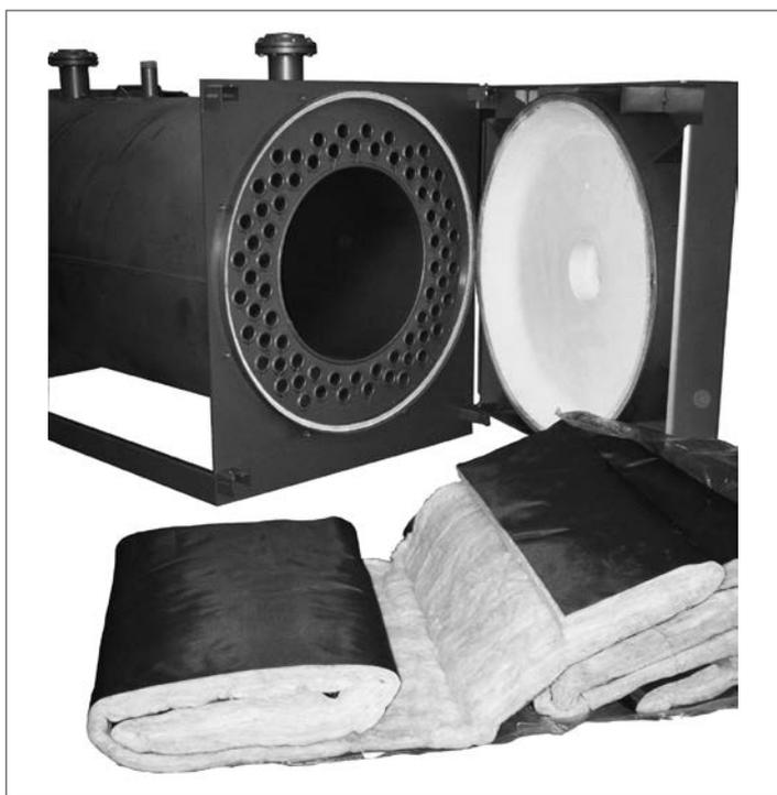
Fit the insulation over the rear of the combustion chamber first, wrapping it around as shown in the figure.
