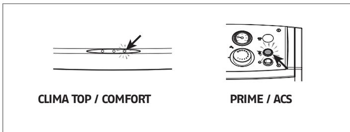
**!** If a "LOCKOUT SHUTDOWN" occurs, wait about 30 seconds before resetting the burner.
