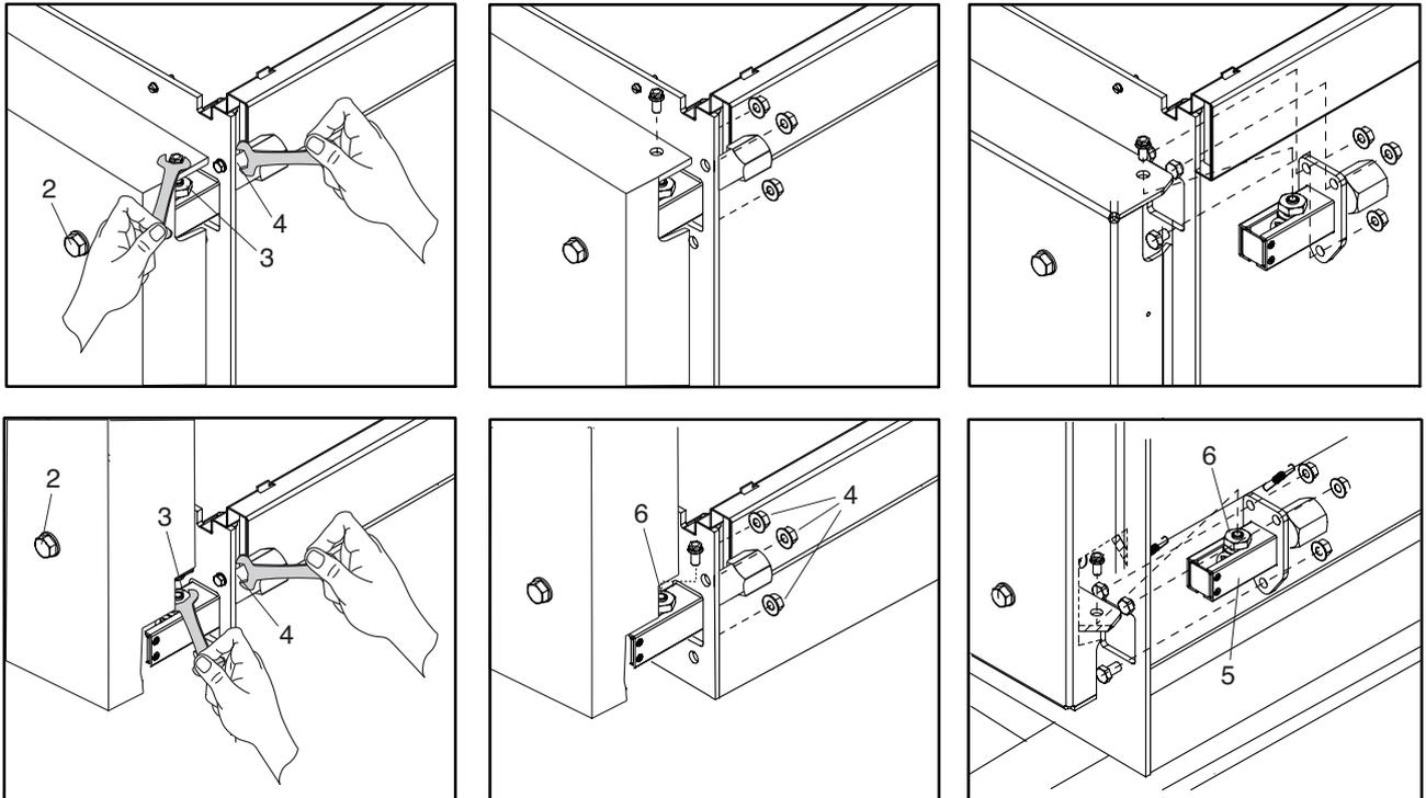
Fit the hinges on the opposite side, making sure that the pivots above the nuts (6) engage the door correctly. If necessary, screw down the nut (6) to raise the pivot. Finally, tighten the bolt (3) to secure the hinge.
