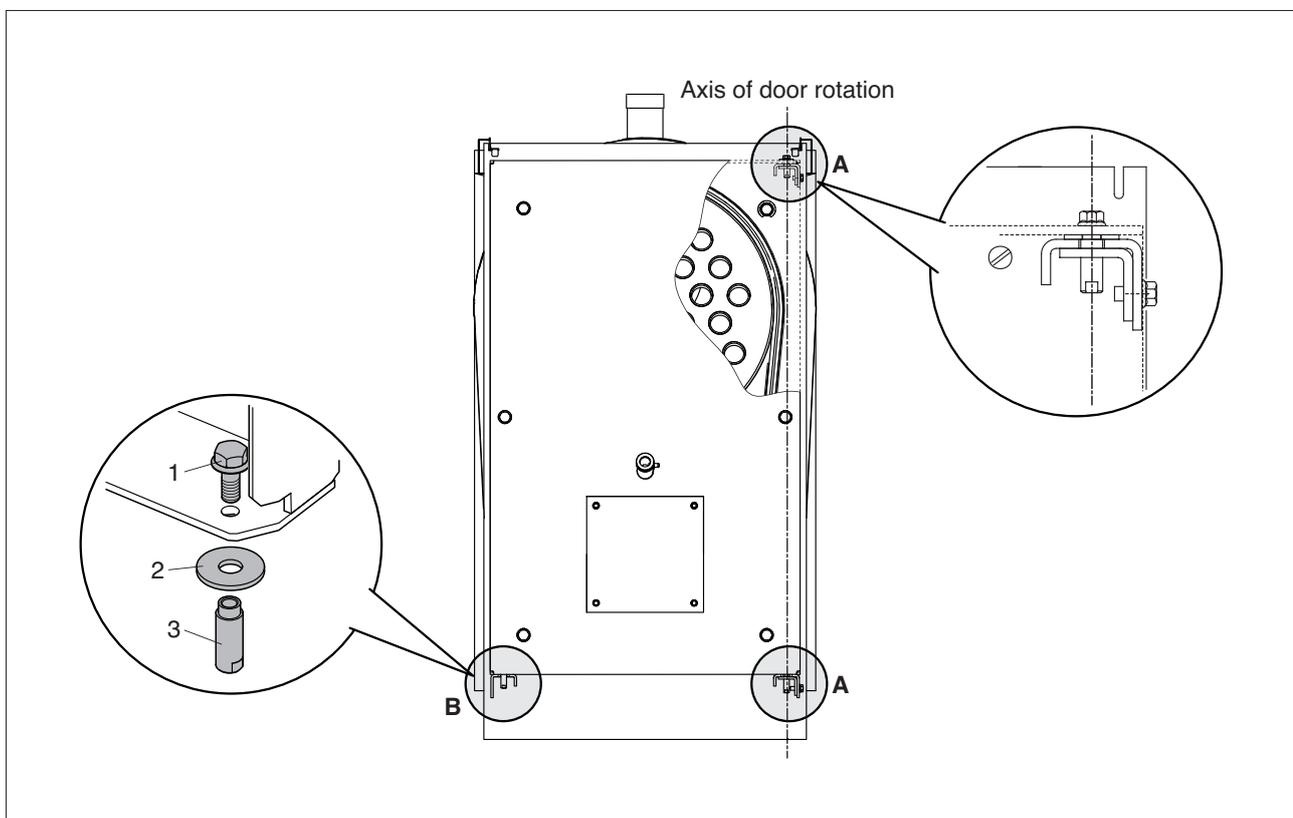
Once you have checked that the default direction of opening is as required, or have reversed the direction of opening as instructed in the '[Changing the direction of door opening](#)' section, remove the spare hinge assembly 'B' (bolt (1), bushing (3) and washer (2)) opposite the hinged side of the door.
