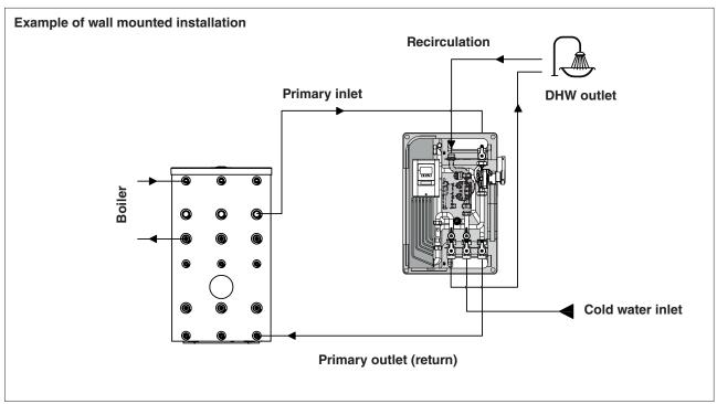
In case of recirculation, provide an expansion tank suitably sized in order to avoid overpressure due to thermal expansion and water hammer.
