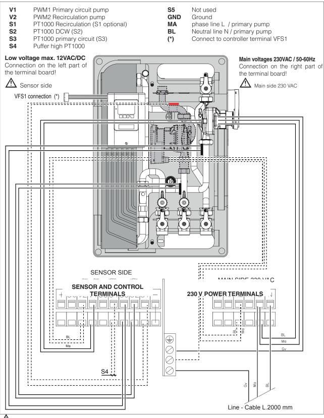
igwedge The polarity of the sensors is freely selectable.
