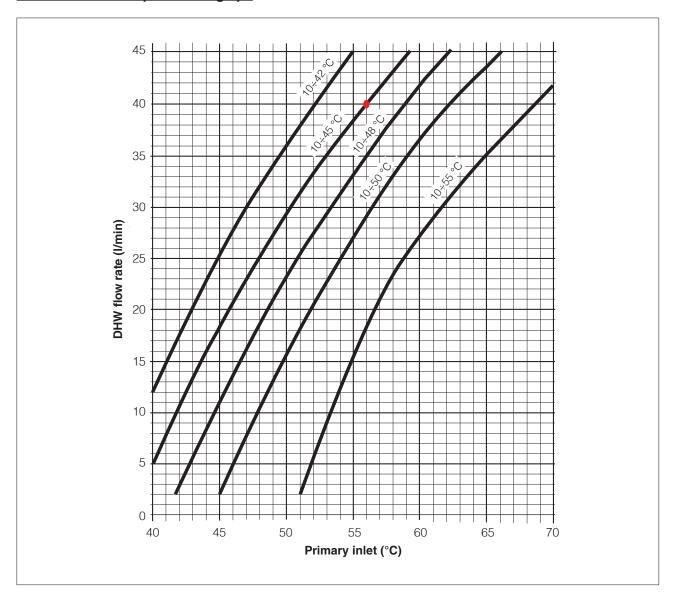
${\bf NB:}$  Correct functioning of the product is only guaranteed if the primary circuit inlet temperature is at least 5°C higher than the DHW setpoint.
