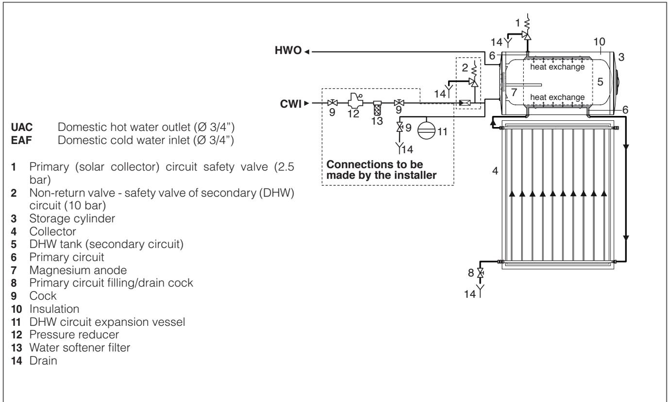
The water supply circuit must permit the storage cylinder to be filled and emptied in safety. Shut-off valves must therefore be easily accessible to the user and the operation of emptying the storage cylinder must not create any risk of flooding or other damage.
