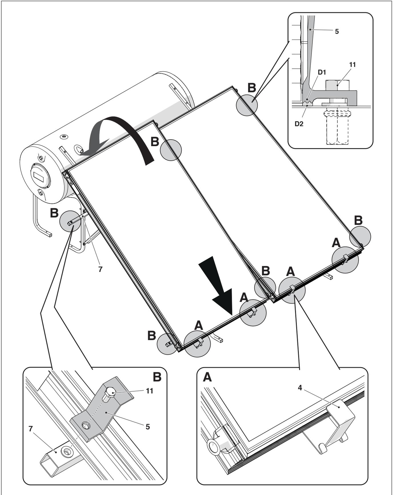
**⚠** Engage the ridges on the clamp (D1) with the ridges on the frame of the collector (D2)
