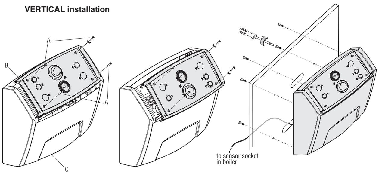
Before you can install the control panel on a boiler side panel, proceed as follows:
