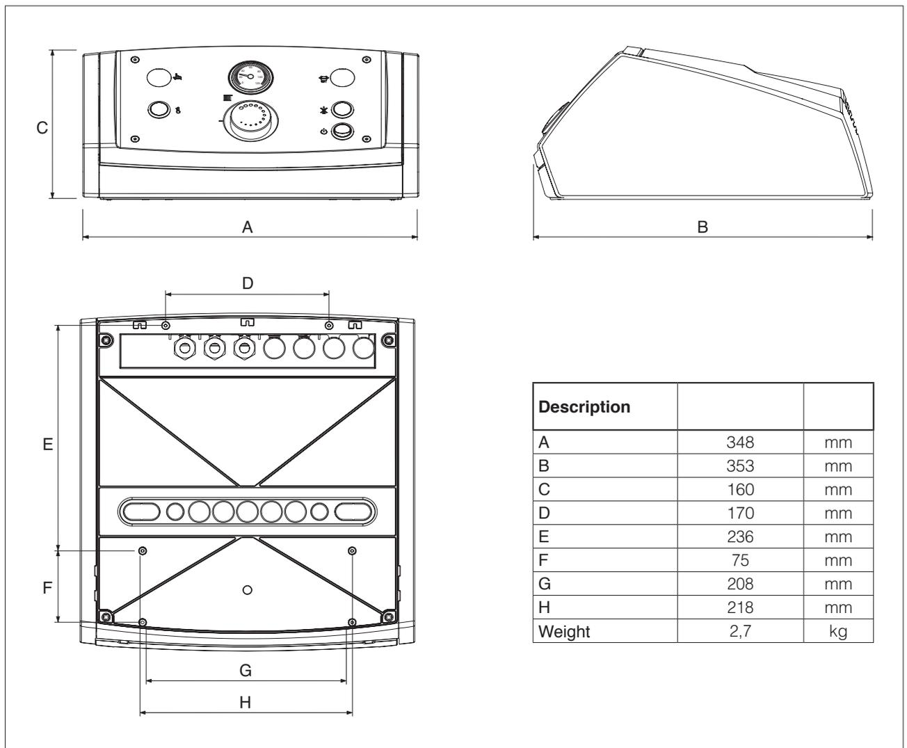
**RIELLOtech PRIME** control panels can be installed either on the top of the boiler or on one of its side panels. Before commencing installation, check the arrangement of the holes on the top panel or side panel of the boiler.
