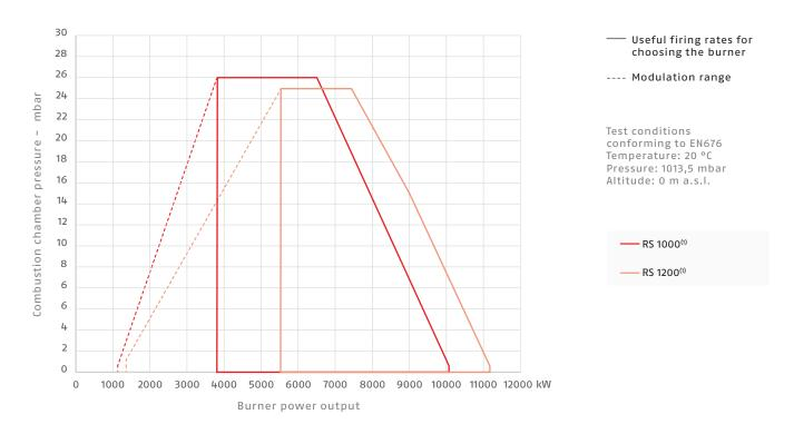
(1) Power range referred to a Low NOx performance conforming to the Class 3 of EN676 European Standard, with 0% of Flue Gas Recirculation; by increasing the recirculation % in order to achieve an Ultra Low NOx emission the burner's maximum output will be reduced
