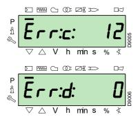
The burner goes into lockout.
