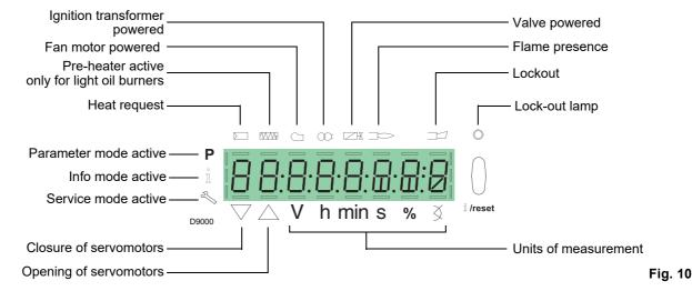
The brightness of the display can be adjusted from  $0 \dots 100\%$  with the parameter 126.
