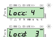
To reset, press the "i/reset" key for 1 s: the display will show "rESEt". When the key is released, the lockout signal will disappear and the red indicator light will switch off.
