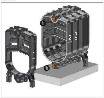
Insert the M16 locking tie-rods into the relative holes and tighten the nuts at the ends to bring the elements closer to each other.
