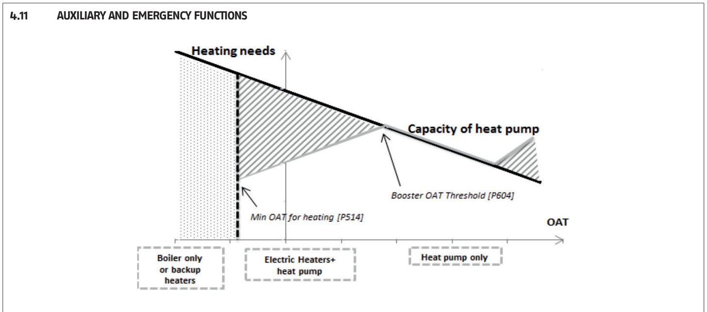
Once the configuration has been completed, it is possible to control up to three electric heaters or three electric heating stages:
