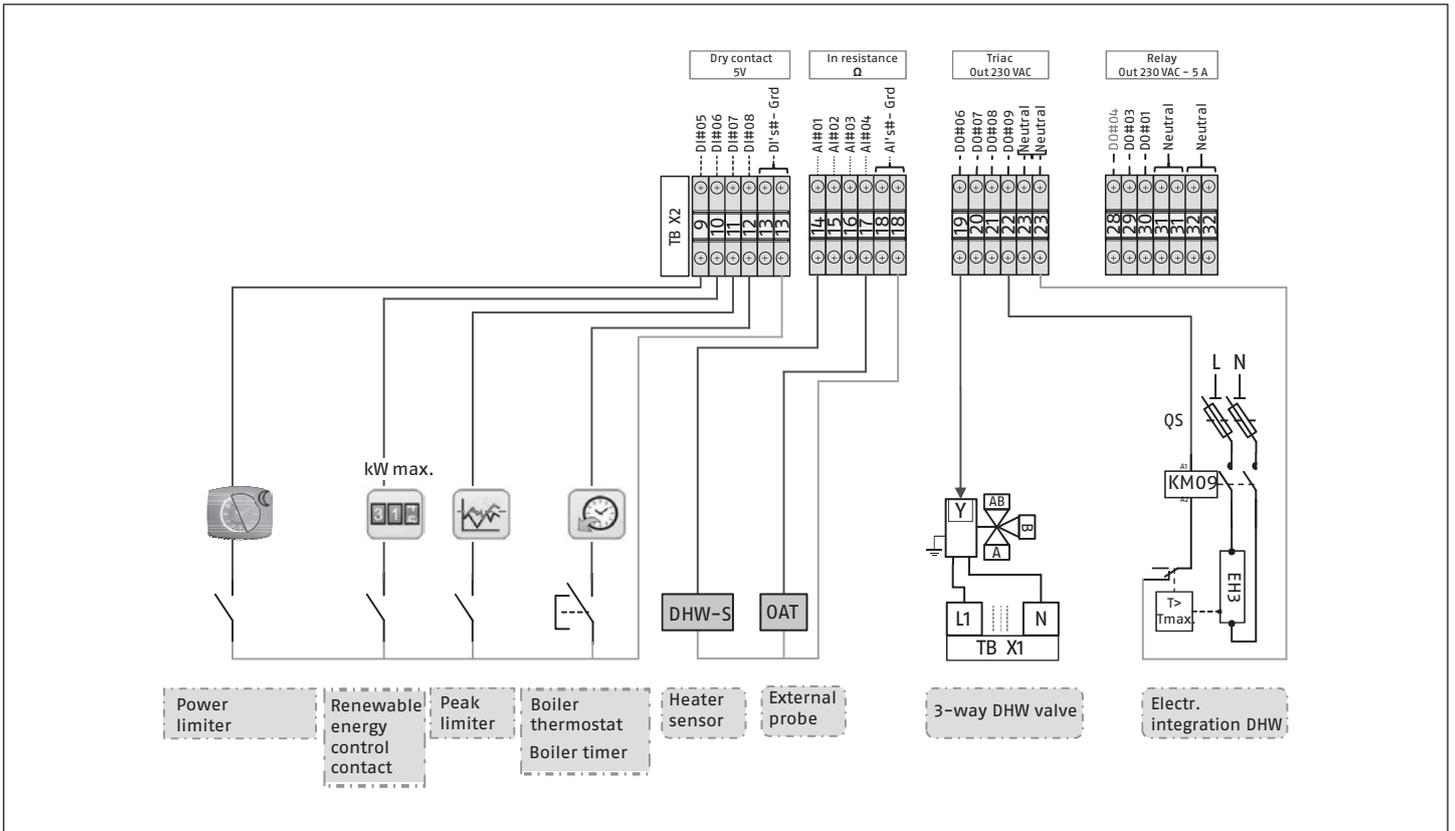
Typical connections for system configurations with heat pump, DHW production and integrated boiler
