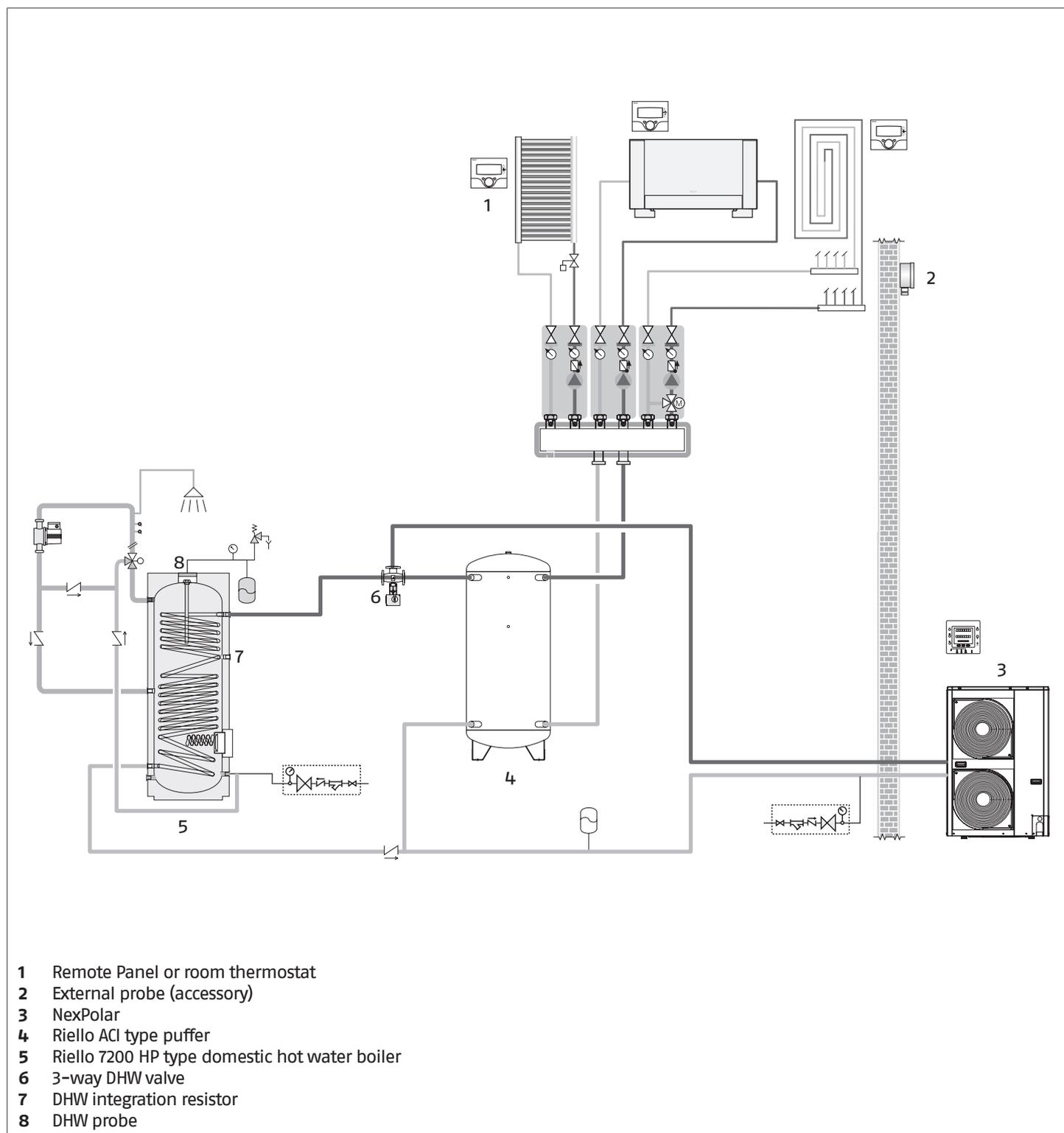
System diagram for heat pump, DHW production and integrated boiler
