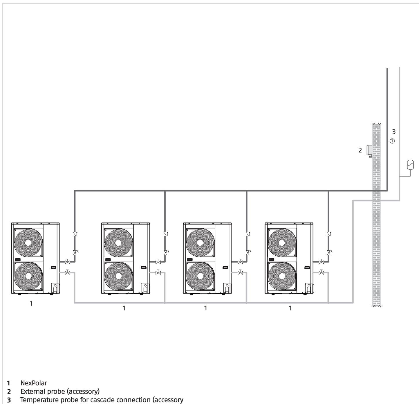
**⚠** Only units of the same model can be connected in cascade configuration.
