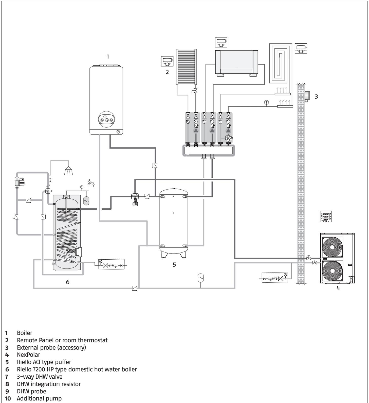
**System diagram for cascade heat pump**
