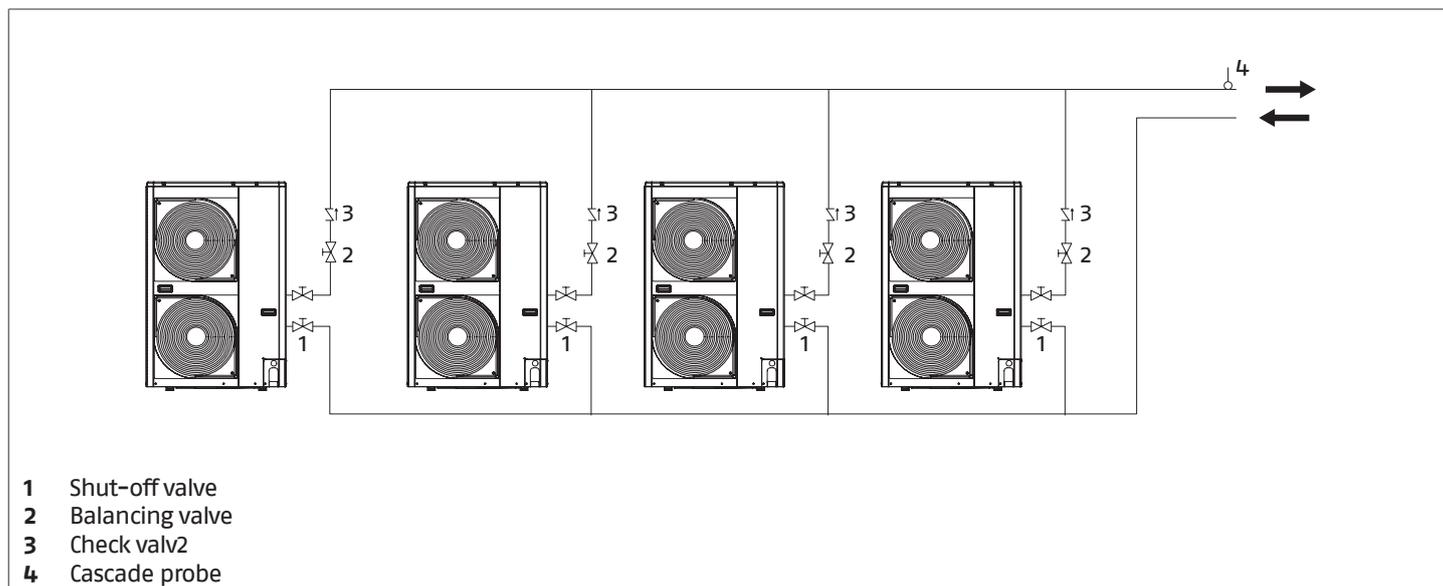
**⚠** Only units of the same model can be connected in cascade configuration.
