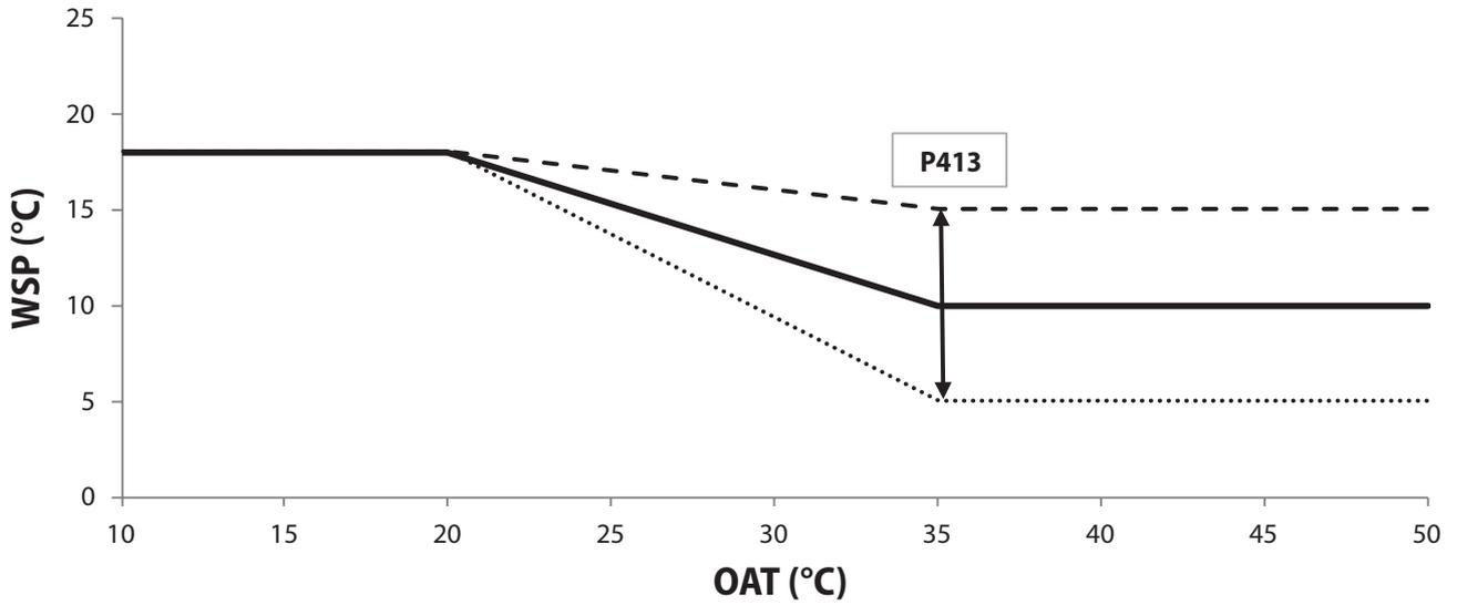
COOLING TEMPERATURE CURVES WITH OFFSETS AT THE TOP
