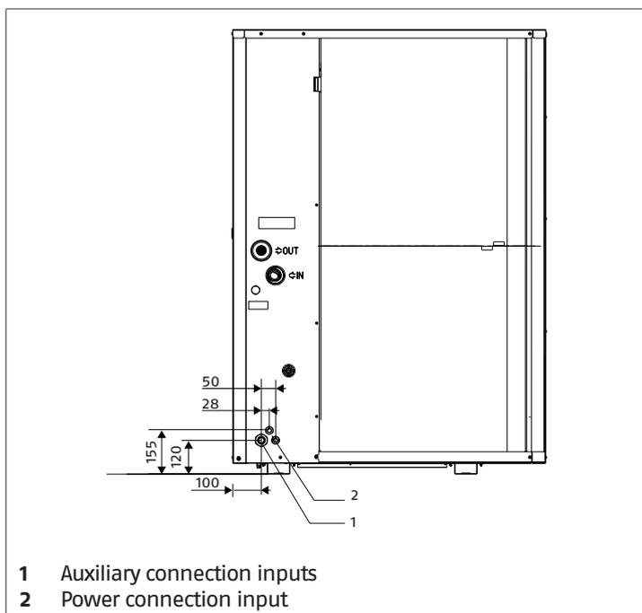
— make electrical connections according to the diagrams here-under.
