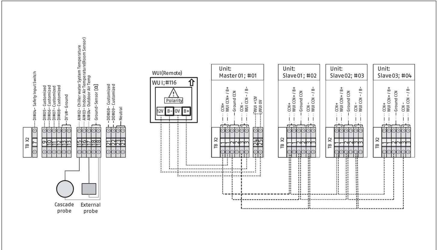
**⚠** Only units of the same model can be connected in cascade configuration.
