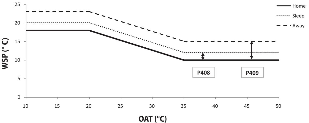
**HEATING:** If the heating temperature curve [P581] is set to "1" or "2", the water setpoint will be calculated based on the selected heating temperature curve.
