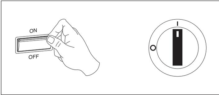
**The device must receive electrical power for at least eight hours before being started up for the first time.**
