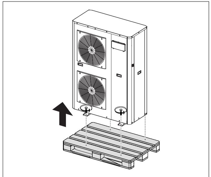
The device is secured to the pallet by 4 screws (two at the front, and two at the back), which must be removed.
