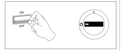
position the system's main switch in the "OFF" position.
