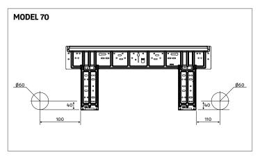
— mark the through hole as shown in the illustration
