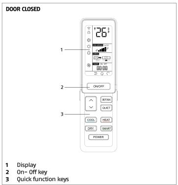
When the door is closed, you can activate the quick functions, such as choosing the operating mode and setting the desired temperature.
