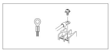
⚠ It is compulsory to use ring crimp terminals to connect to the terminal board.
