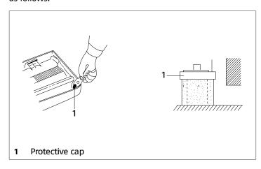
remove the protection plug from the prearranged connection on the right-hand side
