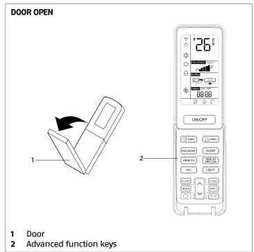
When the door is open, you can access the advanced functions, e.g. time scheduling and motor-driven deflector settings.
