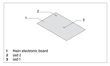
The unit operation is signalled with LED 2.
