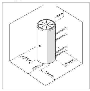
Respect the minimum specified installation distances to ensure correct installation and access for maintenance.
