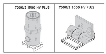
Model Riello 7200/2 2000 HV PLUS are supplied in two separate packages:
