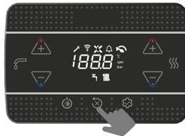
**!** When the venting cycle is running, all heat requests are inhibited apart from DHW unless the boiler is OFF.
