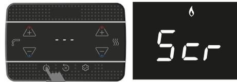
Once activated, this function takes maximum priority. If there is a power failure and reset, the function will resume from the point where it was interrupted.
