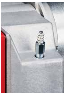
Air damper adjustment
