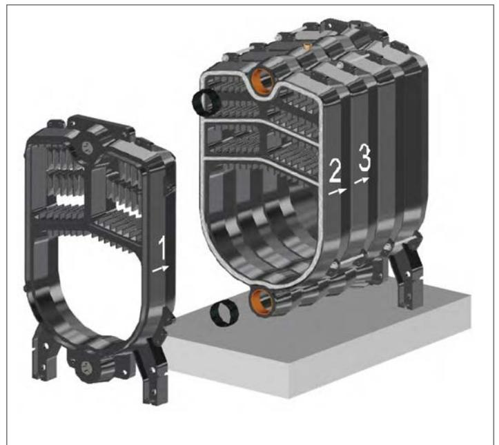
Insert the M16 locking tie-rods into the relative holes and tighten the nuts at the ends to bring the elements closer to each other.
