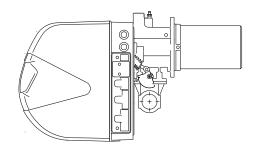
Progressive two-stage or modulating gas burners with electronic cam, with low NOx emissions according to Class 5 of European standard EN 676 (NOx lower than 56 mg/kWh)
