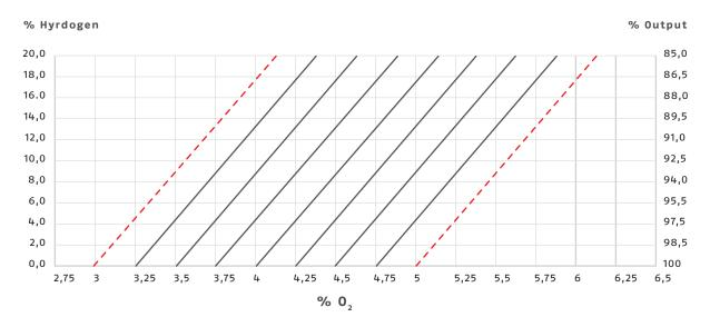
Adjusting the burners as suggested makes them ready for injections of hydrogen into the natural gas grid without the need for further settings, up to the maximum hydrogen value of 20%, as certified according to the boundary conditions defined in DVGW CERT ZP 3502 edition 01.12.2022.
