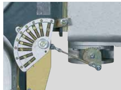
Example of the variable profile cam on RS 250/M MZ burners.
