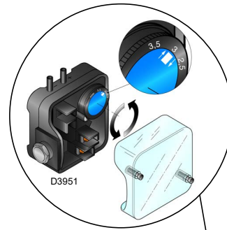
Connection of the pressure gauge with the pressure switch in absolute
