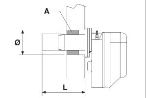
When you finish installing the burner in the boiler, fill the gap between the burner's blast tube and the refractory material in the door with the ceramic insulation (A) supplied with the boiler.
