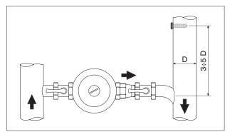
A sensor socket must be positioned at a distance of 3 to 5 times the diameter of the water return pipe, upstream from the water fitting, to measure effective water return temperature and control the anti-condensate pump or the temperature controller stabilisation function.
