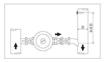
$\triangle$  A sensor socket must be positioned at a distance of 3 to 5 times the diameter of the water return pipe, upstream from the water fitting, to measure effective water return temperature and control the anti-condensate pump or the temperature controller stabilisation function.
