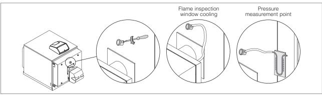
A rubber socket is attached to the flame inspection window. If this is used as a pressure measurement point, leave the screw in place in order to close off the pressure measurement line during normal boiler functioning. If the rubber socket is used to cool the flame inspection window, remove the screw to ensure an adequate air flow.
