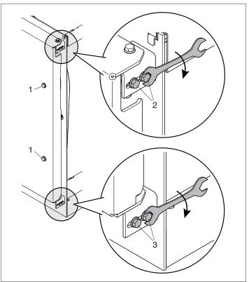
A Make sure that the door is properly adjusted after every maintenance operation.
