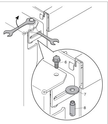
fit the bushing (8), bolt (6) and washer (7) to the opposite \_ side of the door.
