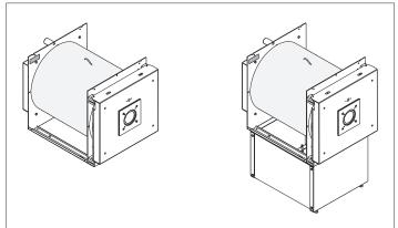
If you are installing the boiler without a pedestal, the limited gap between the burner and the floor makes it particularly important to keep the boiler room clean.
