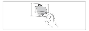
Provided all the above conditions are satisfied, start the boiler up again, then analyse the combustion fumes, measure fuel flow and re-check the door seal.
