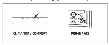
A If a "LOCKOUT SHUTDOWN" occurs, wait about 30 seconds before resetting the burner.
