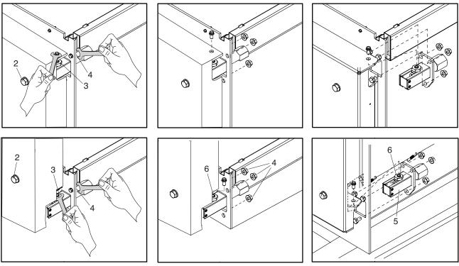
Fit the hinges on the opposite side, making sure that the pivots above the nuts (6) engage the door correctly. If necessary, screw down the nut (6) to raise the pivot. Finally, tighten the bolt (3) to secure the hinge.
