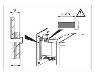
See the instruction manual provided with the burner for further information on burner installation, electrical connections, burner adjustments. If a two stage burner is installed, 1<sup>st</sup> stage heat input must not be less than 70% of total heat input.
