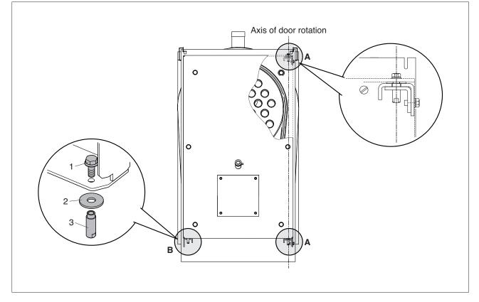
Once you have checked that the default direction of opening is as required, or have reversed the direction of opening as instructed in the '<u>Changing the direction of door opening</u>' section, remove the spare hinge assembly 'B' (bolt (1), bushing (3) and washer (2)) opposite the hinged side of the door.
