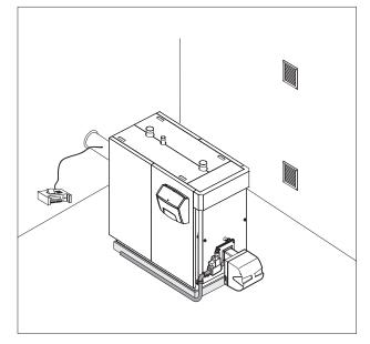
Provided all the above conditions are satisfied, start the boiler up again, then analyse the combustion fumes, measure fuel flow and re-check the door seal.
