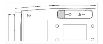
If a "LOCKOUT SHUTDOWN" occurs, wait about 30 seconds before resetting the burner.
