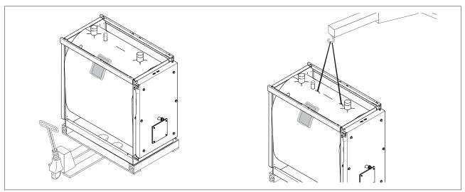
$\triangle$  When moving the boiler, take particular care not to damage the front panel.
