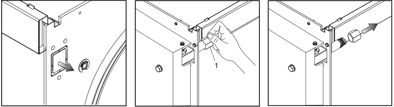
Open the door and use a hacksaw or file to remove the cutout from the front head on the opposite side to the door hinges. Reclose the door and secure it with the bolts (2). Remove the plug (1), taking care not to lose the spring from inside the threaded tube.
