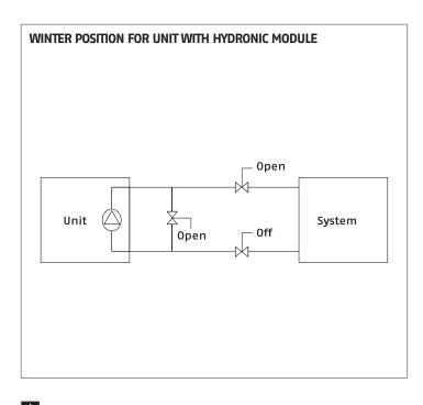
A When the unit switches to winter mode, based on the local atmospheric conditions, it is necessary to do the following:
