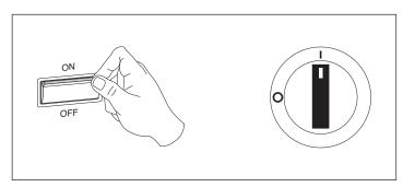
The device must receive electrical power for at least eight hours before being started up for the first time.
