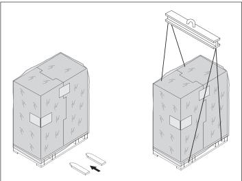
It should be noted that, even if the user decides to use a forklift or pallet jack, a hoist or crane will nevertheless be required in order to remove the **RIELLO NexPolar** unit from the pallet and position it in the foreseen place of installation.
