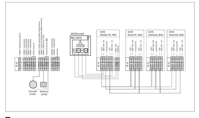
Only units of the same model can be connected in cascade configuration.
