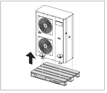
The device is secured to the pallet by 4 screws (two at the front, and two at the back), which must be removed.
