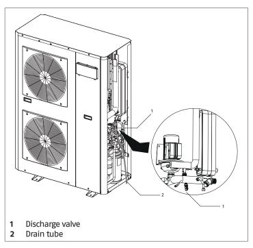
close the discharge valve once the operation has been completed
