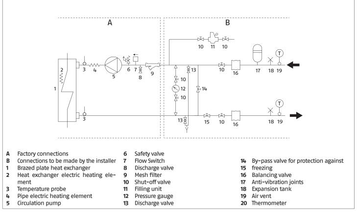
The water connections must be completed by installing:
