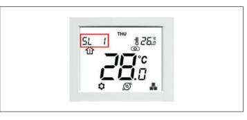
— press V or A to select Slave unit no.2 - change according to the following table
