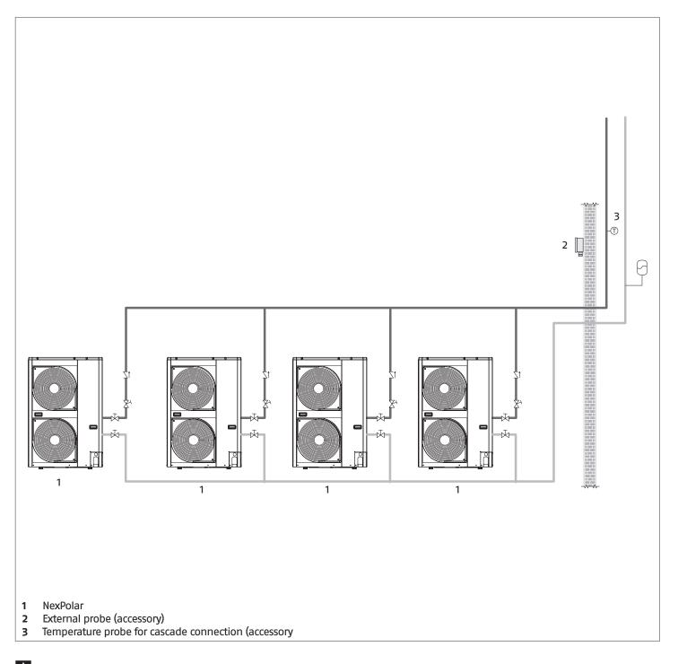
• Only units of the same model can be connected in cascade configuration.
