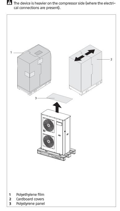
🗴 The device must always be handled and moved in an upright
