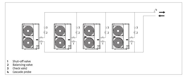
• Only units of the same model can be connected in cascade configuration.
